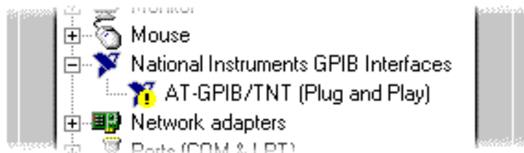
Figure C-1. GPIB Interface That Is Not Working Properly
