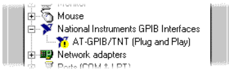
Figure 2-6. GPIB Interface That Is Not Working Properly
